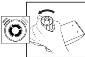
2. Remove the water tank and turn the tank upside down – remove the tank cap by turning it counter-clockwise.
