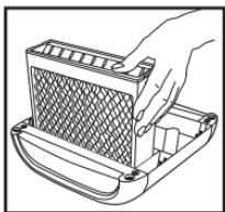
1. Be sure the Cooling Media is positioned with the "V-shaped" vents facing upward. **Never operate the unit without the cooling media.**
