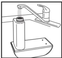
3. Fill the water tank with clean, cool (not cold) water. We recommend using distilled water if you live in a hard water area. **Never use any additive or place essential oils into the water. Even a few drops will damage the unit.**
