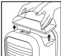
1. Unplug the Power Adaptor from the wall and from the unit. Remove the water tank from the top housing.
