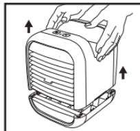
2. Gently lift and remove the Top Cover from the Personal Space Cooler. Pour out any excess water remaining in the Water Reservoir.
