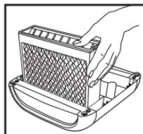
4. Set the new Cooling Media in place. Be sure the Cooling Media is positioned with the "V-shaped" vents upward.
