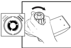
4. Replace the tank cap by turning clockwise until tight. Do not overtighten.
