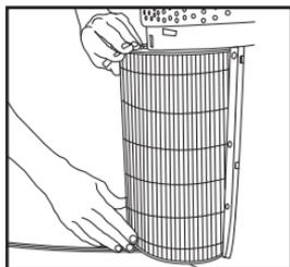
4. With the filter tabs facing outward, insert the new True HEPA filter.
