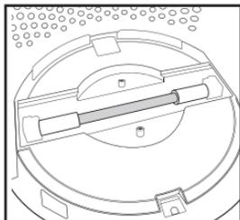
2. Remove the cover to expose the UV-C bulb.
