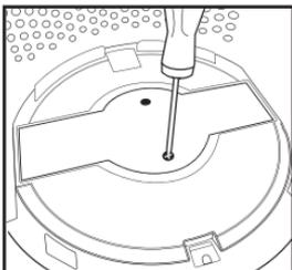
1. Unplug the air purifier and remove the True HEPA filter. Using a Phillips-head screwdriver (not included), unscrew the 2 screws located on the UV-C bulb cover.
