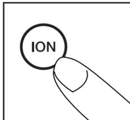
6. Plug the power cord into a standard AC outlet and press the power
