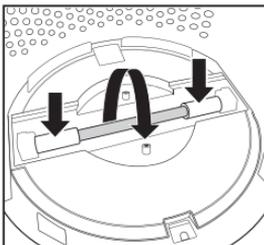
3. Gently push from the sides and rotate the UV-C bulb to remove.
