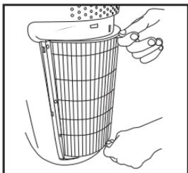
3. Pull the tabs to remove the old filter.
