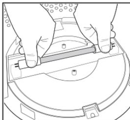
4. Remove and replace the UV-C bulb. Re-install the UV-C bulb cover, True HEPA filter, and grille cover.
